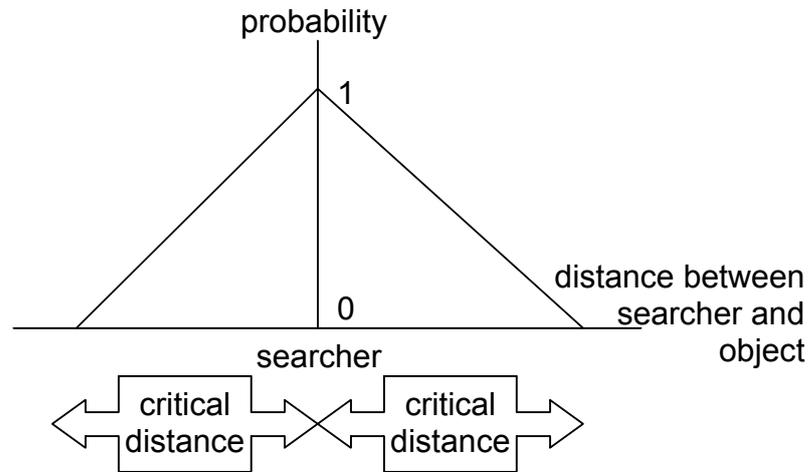
Figure 1: the linear lateral range curve (LLRC)
